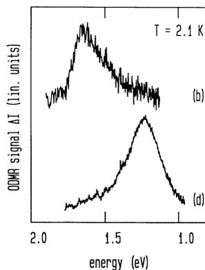
Fig. 3. Spectral dependence of the donor ODMR signals for (b) the starting material LEC GaP:S annealed (800°C, 1 h) and (d) irradiated and subsequently annealed (800°C, 1 h). Spectra are measured at 2.1 K with a 1.5 m monochromator and a Ge detector.
