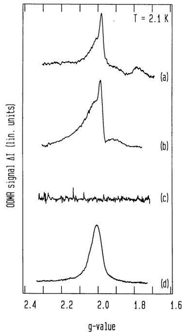
Fig. 2. ODMR spectra measured at 2.1 K of (a) the starting material LEC GaP:S, (b) annealed (800°C, 1 h), (c) as-irradiated and (d) irradiated and subsequently annealed (800°C, 1 h). Changes of the total infrared emission ( $\Delta I$ ) under 514.5 nm  $\text{Ar}^+$  excitation are plotted against  $g$ -value.
