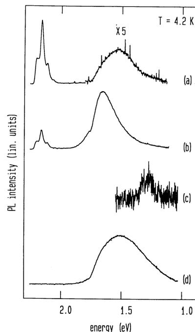
Fig. 1. PL spectra measured at 4.2 K of (a) the starting material LEC GaP:S (b) annealed (800 °C, 1 h), (c) as-irradiated and (d) irradiated and subsequently annealed (800 °C, 1 h). Spectra are measured under 514.5 nm  $Ar^+$  excitation with a 1.5 m monochromator and a Ge detector.
